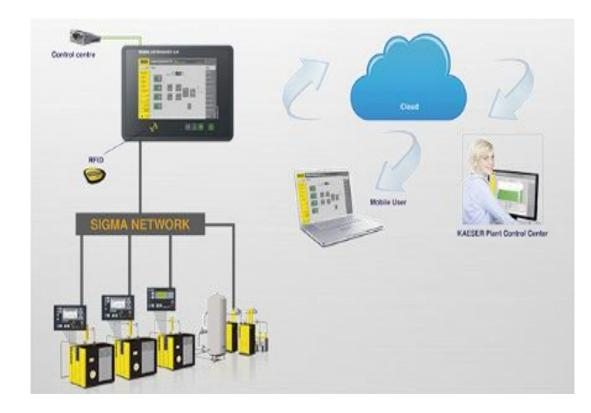
Sigma Air Manager 4.0 is the core of the compressed air station and provides the key technology required to take advantage of future services within the Industry 4.0 operating environment. As the central "brain" of a compressed air system, it assumes control tasks and streams data into the Kaeser Data Center. This master controller opens up new possibilities to enable predictive maintenance of compressors.
